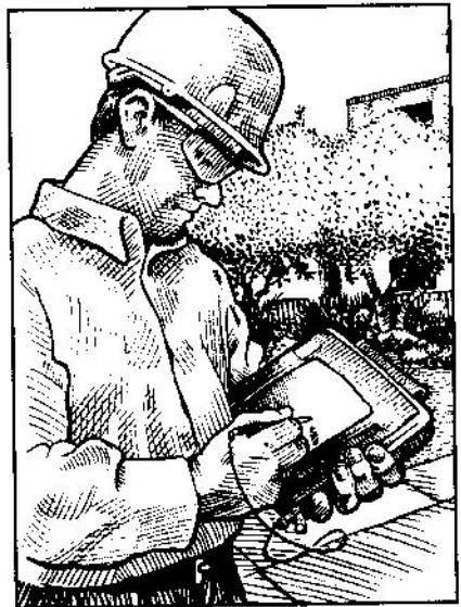
A data collector using a pen-based unit to record tree location on a geo-rectified map. The collector also gathers information about species, diameter, and other attributes.
