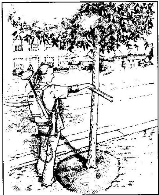
A data collector carrying a GPS unit on her back for establishing tree location and using a Biltmore stick to measure tree diameter.
